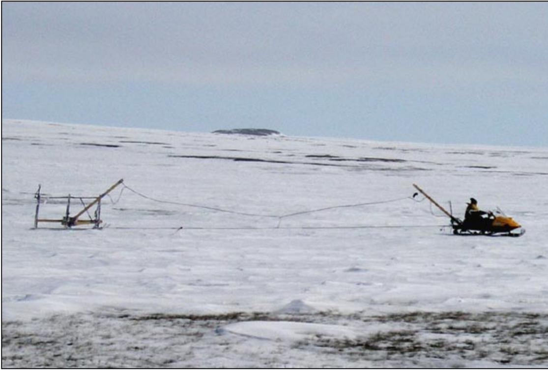
JVX ROVER snowmobile magnetometer system surveying one of the target areas.
