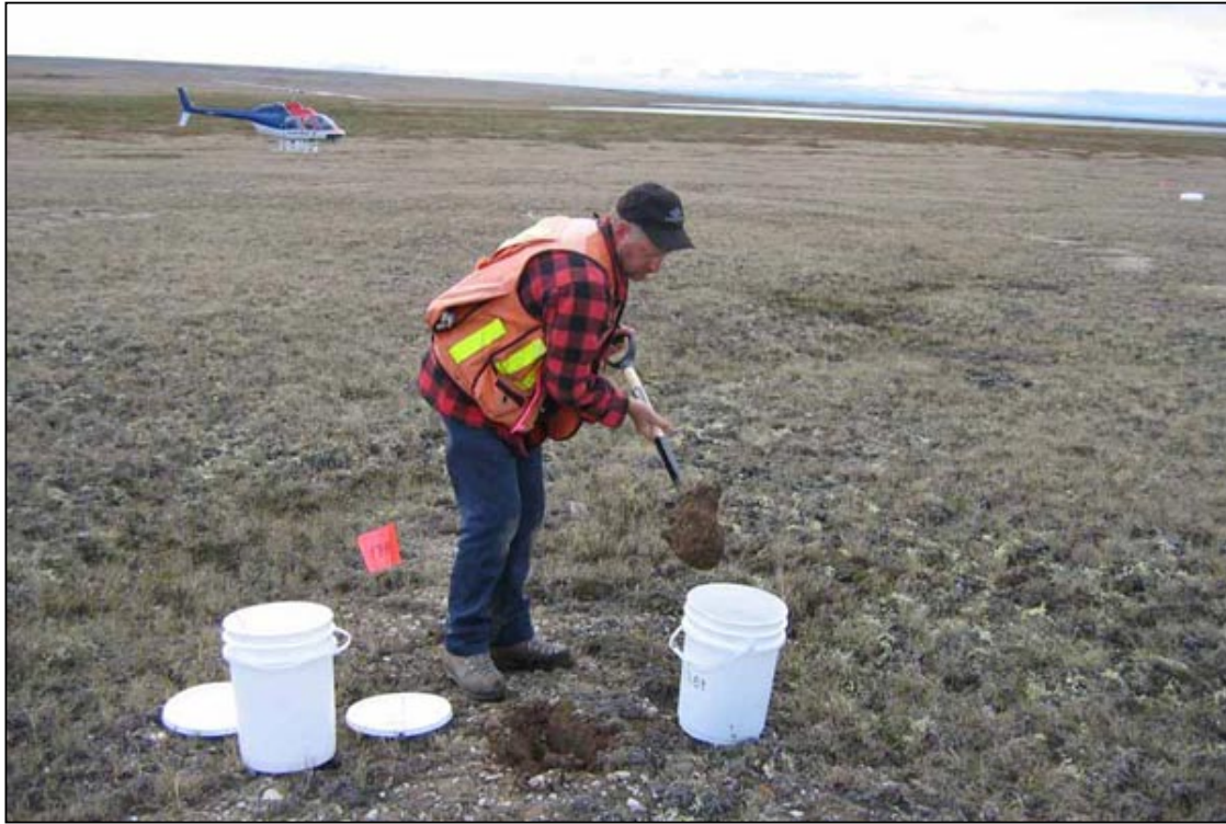
Tim Sandberg, Taiga Consultants Senior Geologist taking a till sample on Parry Peninsula.
